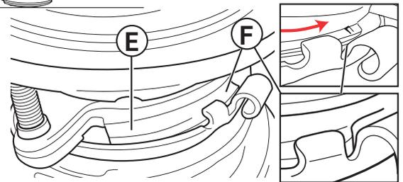
As the Lower Mount Ring is turned counter clockwise each tab slides up onto the Upper Mount Ring Ramp (E) and locks in position over the Ridges (F).
