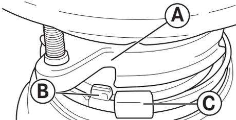
The lower mounting ring (which is part of the disposer) has 3 tabs that grab the mounting ring ramp.
