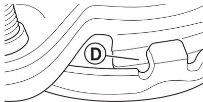
Lift and turn the Lower Mount Ring counter clockwise until all three mount tabs lock over the Ridges (F) on the slide-up Ramps (D) of the Upper Mount Ring.
