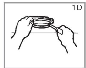
**Caution:** Be sure to support the disposer while performing this step or it may fall when the mounting ring is disconnected from the mounting assembly.
