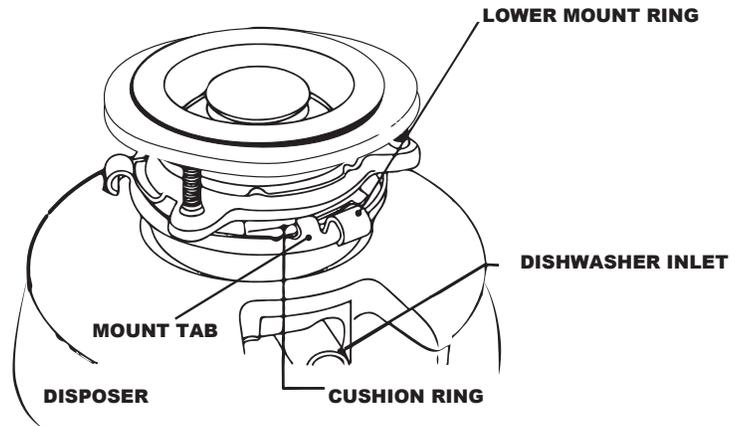
**NOTE: Cushion Ring included between the Upper Mount Ring and Lower Mounting Ring.**
