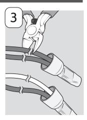
3. Using wire cutters, cut black (or brown) wire and white (or blue) wire near the connectors.
