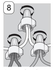
8. Connect disposal wire leads (black and blue) to corresponding wire leads of the power supply cable. Green always connects to green.
