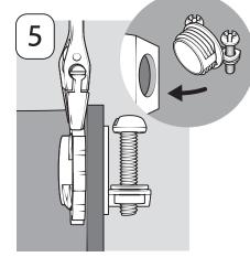
5. Insert metal strain relief connector (not included) into the endbell hole and tighten the nut securely.
