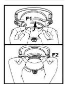
F. Hold the three parts in place while attaching the Retainer Ring (F1) by pulling it apart and having it snap within the groove of the sink flange (F2).
