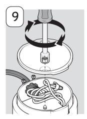
9. Setting the wires into the endbell, replace the end plate and tighten the two bolts.
